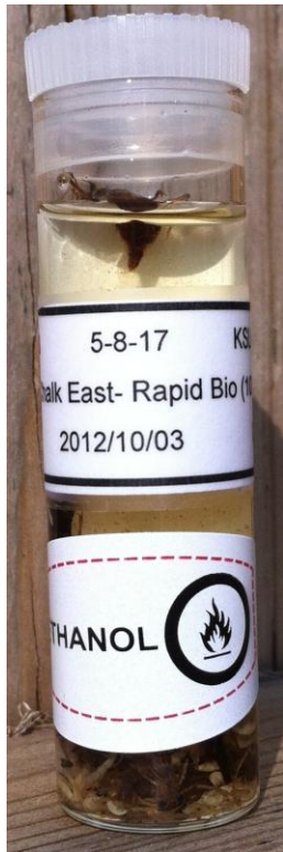
Figure 2. DESC-style vial for archiving a benthic-invertebrate sample, showing mandatory sample-metadata and WHMIS labels (this example is borosilicate glass shell vial, manufactured by Fisherbrand™)
