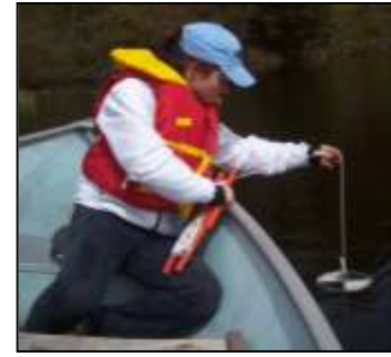
Above: A Secchi disk is used to measure water clarity in a lake.
