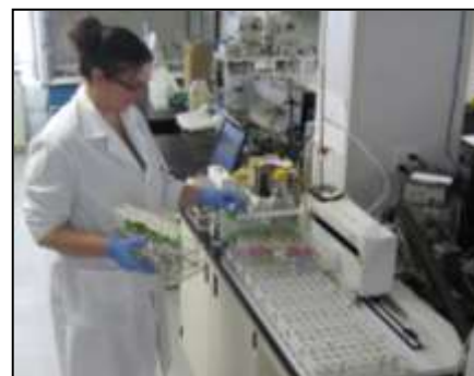
Above: Chemistry Technician at the Dorset Environmental Science Centre performs total phosphorus analyses on Lake Partner Program water samples.
